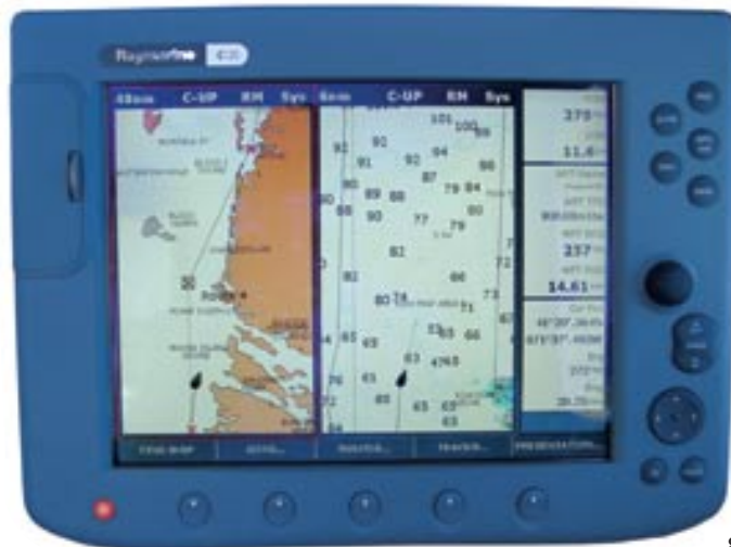
The C120 offers excellent control of chart windows, as well as custom display pages.
